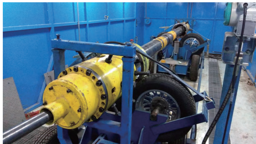
Figure 4 Full scale fatigue test
